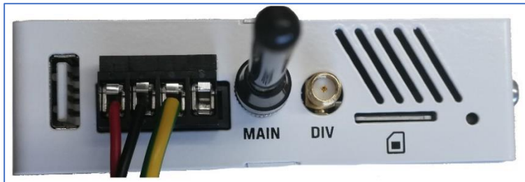
Screenshot 7 RAR with mobile phone option: 3G/4G antenna installed on the SMA connector of the mobile device.
