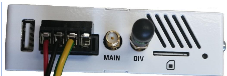
Screenshot 8 RAR with WIFI antenna installed on the SMA connector for the 2.4 GHz signal.
